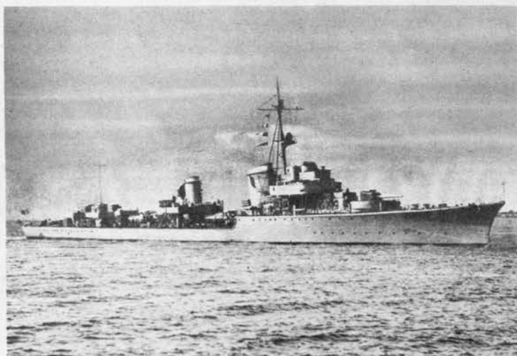
NARVIK CLASS is Germany's finest, mounts four or five very big guns, up to 5.9-in., they probably exceed designed speed of 36 knots.
